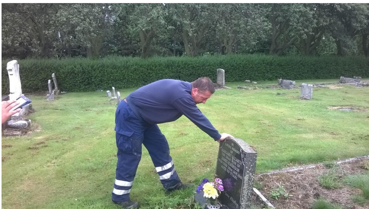
Example of staff carrying out a gentle hand test up to 25KG
