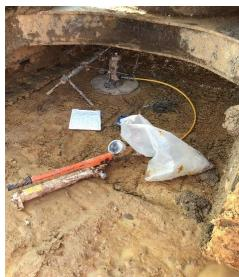
Stone compaction testing and plate bearing tests were undertaken on the piling platform.
