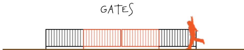
A minimum of two gated access points are required for all fenced play spaces, typically: a single leaf flat top hydraulic self-closing pedestrian gate; and a double leaf, combined flat top hydraulic self-closing pedestrian gate and maintenance gate. All gates to be finished in a high contrast colour, such as red or yellow.
