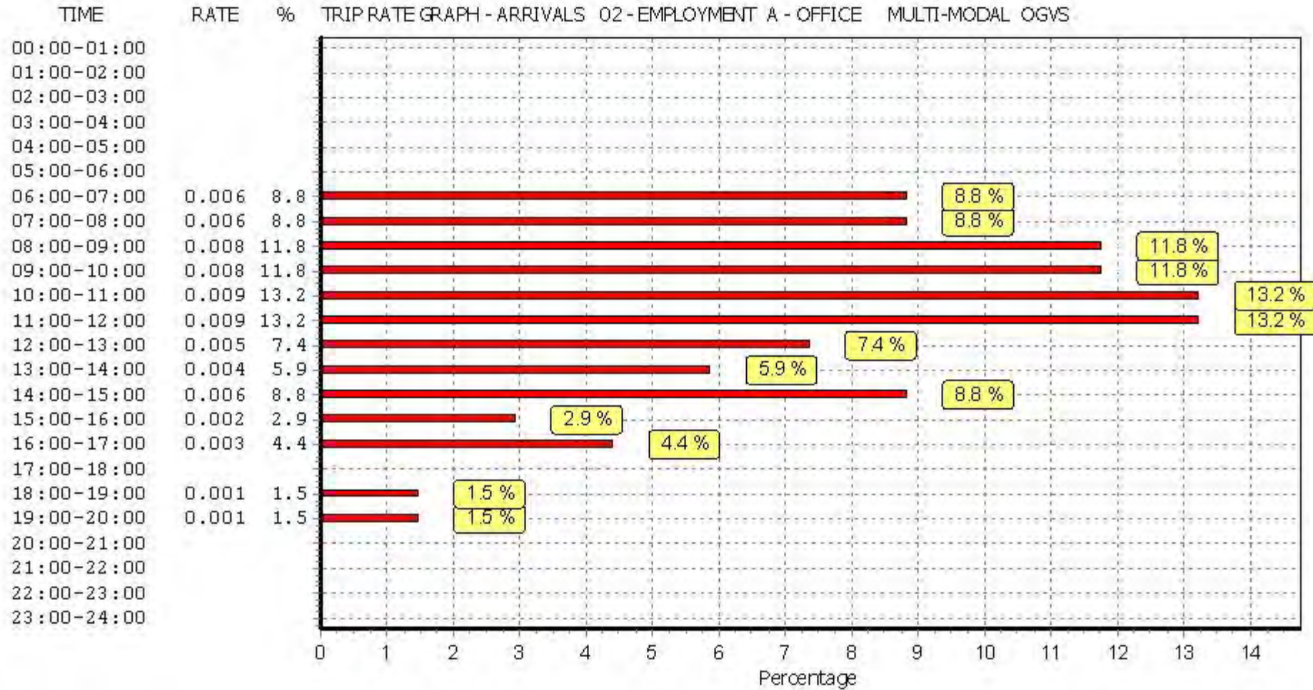
This graph is a visual representation of the trip rate calculation results screen. The same time periods and trip rates are displayed, but in addition there is an additional column showing the percentage of the total trip rate by individual time period, allowing peak periods to be easily identified through observation. Note that the type of count and the selected direction is shown at the top of the graph.
